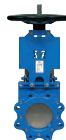
Series 702/20 Knife gate valve with handwheel and rising stem DN50-1200 PN10 Ductile iron Options: • handwheel and non-rising stem • chainwheel • electric or pneumatic actuator • lever
