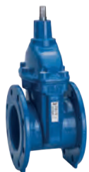
Series 06/80 Flanged gate valve Face-to-face DIN F4 DN40-600 PN10/16 NBR wedge Ductile iron Options: • AISI 316 stem • face-to-face DIN F5
