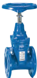
Series 06/35 Flanged gate valve with position indicator Face-to-face DIN F4 DN50-400 PN10/16 EPDM wedge Ductile iron Options: • NBR wedge • face-to-face DIN F5 • OS&Y
