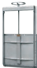
Series 772/61 Wall penstock Bi-directional up to and incl. 1200 x 1200 mm, in larger sizes bi- or uni- directional With non-rising stem Stainless steel AISI 304 200 x 200 mm - 2000 x 2000 mm Options: • rising stem • AISI 316
