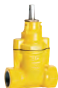
Series 03/25 Service connection valve with internal thread DN25-50 PN4 Ductile iron External epoxy coating
