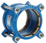
Series 621/10 Supa Plus™ coupling Tensile for PE and uPVC pipes DN32-300 PN16 Ductile iron
