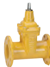
Series 02/70 Flanged gate valve Face-to-face DIN F5 DN40-500 PN10/16 Ductile iron External epoxy coating
