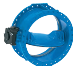
Series 756/106 Butterfly valve Double eccentric Double flanged Welded stainless steel seat IP 68 gearbox DN150-1400 PN10/16 Ductile iron
