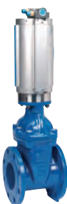
Series 715 Flanged gate valve with hydraulic actuator Face-to-face DIN F4 DN65-300 PN10/16 NBR wedge Ductile iron Options: • solenoid valve kit and proximity switches
