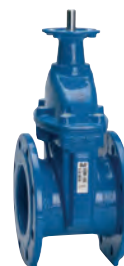
Series 15/42 Flanged gate valve for electric actuator Face-to-face DIN F4 DN40-400 PN10/16 Ductile iron Options: • face-to-face DIN F5 • hydraulic/pneumatic actuator • NBR wedge
